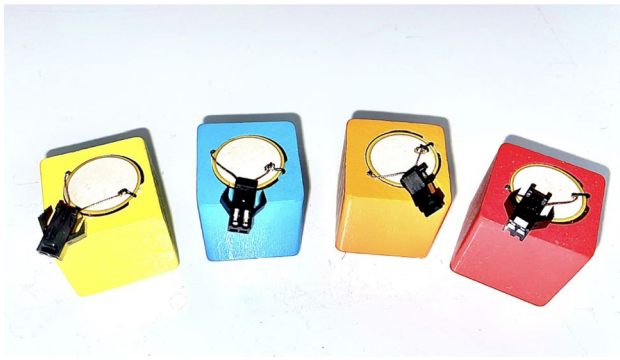
Fig. 12 2.0 cm wooden cubic blocks per side with acoustic marker
